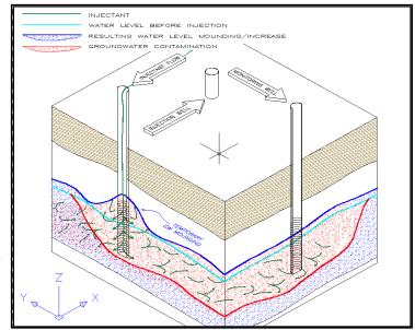
In the second pipeline location, Exo Tech performed a more comprehensive injection in October 2011 that consisted of approximately 20,500 pounds of iron activated persulfate delivered into 135 points. Treatment goals in this location were to reduce dissolved BTEX to
